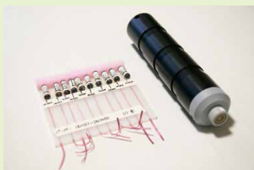
Pinger ultrasonic tag and receiver The receivers can detect signals from tagged fish in a 500-meter radius and provide nearly real-time observation.
