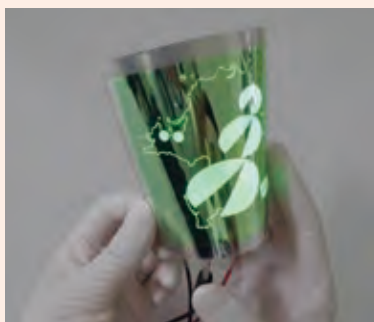
OLED devices made with AEF are also bendable *This technology is being co-developed with the Institute of Systems, Information Technologies and Nanotechnologies
