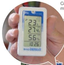
Compact WBGT heat-stress measurement device
