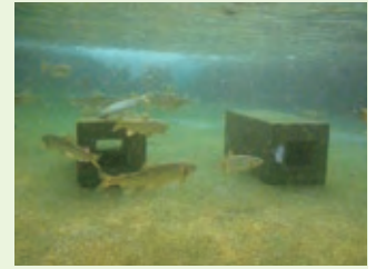
“Organic concrete” (left) attracts more fish than conventional concrete (right).
